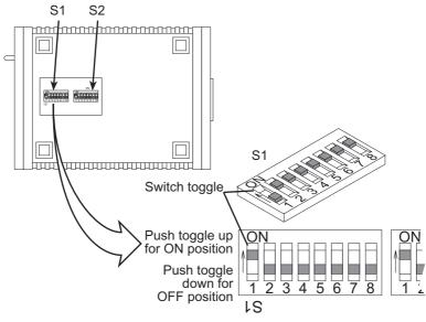
Figure 3. DIP switches S2 and S2
